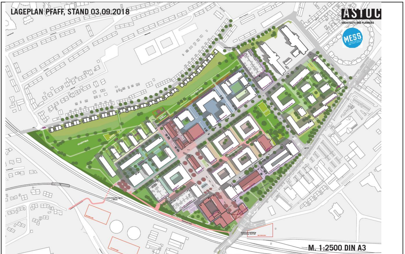
Plan of the Pfaff-Quarter with existing buildings, which will be refurbished (red) and planned new buildings (white)
