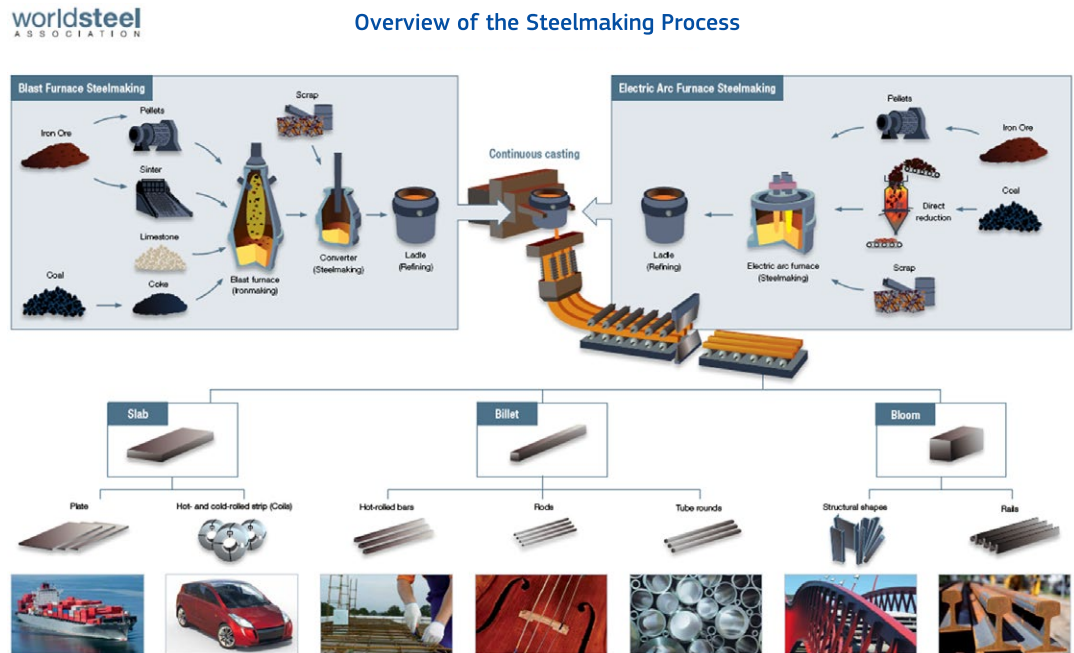
Figure 20.3: Overview of the steel- making process and variety of products manufactured
