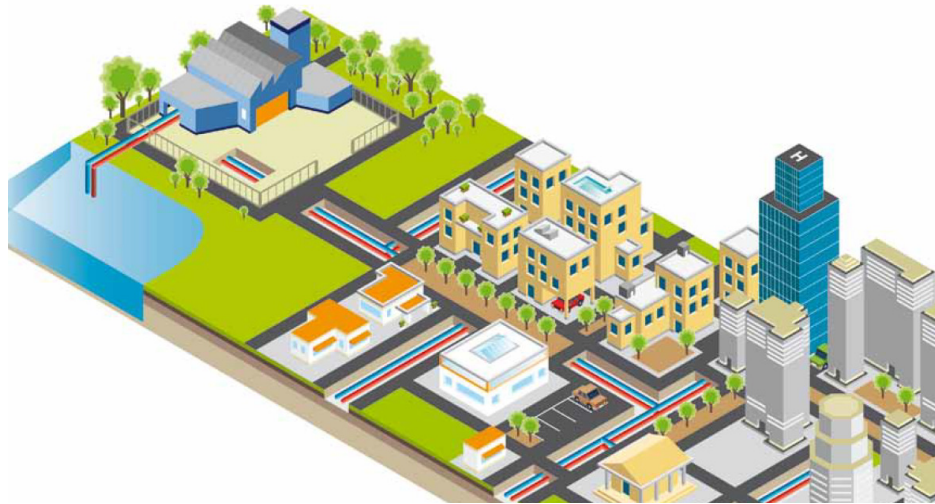
Figure 14: Illustration of a district cooling system (ref. /27/)
