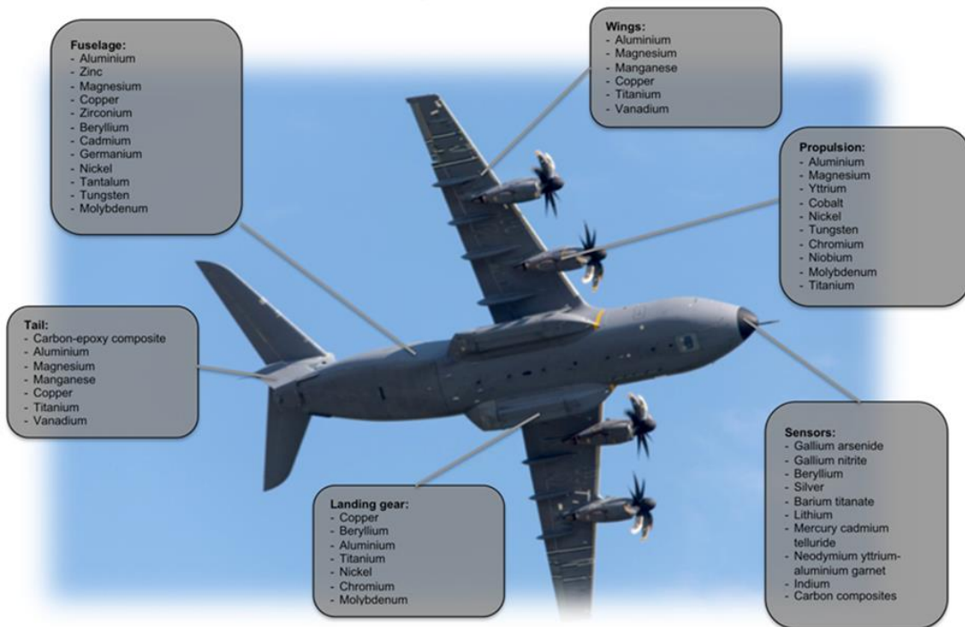
Figure 3.2: Components and raw materials used in different parts of the transport aircraft A400M produced by Airbus D&S (source: CEIS)
