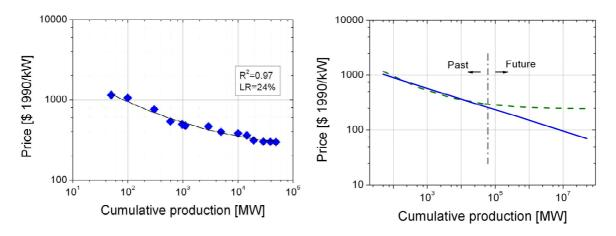
Figure 3: Multi-component learning for gas turbines (left) and implications for future predictions
