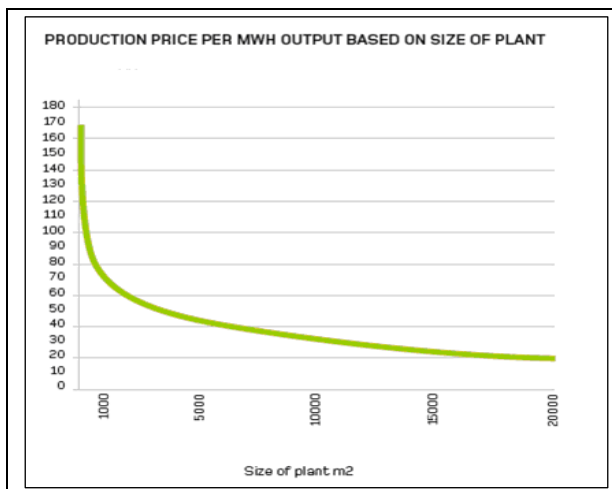
Figure 9-6 The cost of solar district heating falls off with increasing size 102
