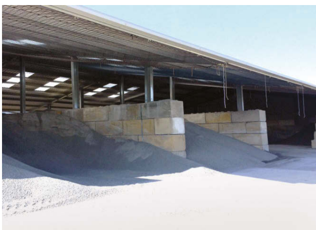
Figure 3: Stock-piled carbonated manufactured aggregate at Carbon8's Suffolk plant
