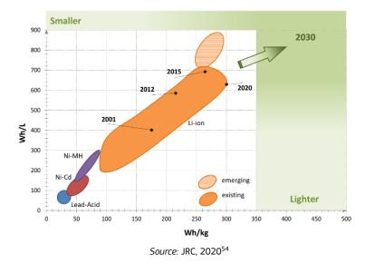
Figure 21. Energy density of Li-ion batteries at cell level over recent years.
