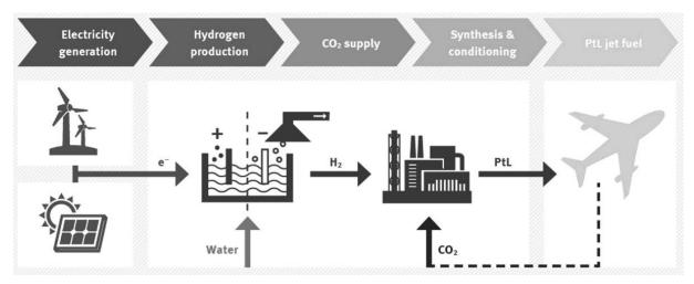
Figure 1. Generic scheme for PtL production (source Schmidt et al., 2018)
