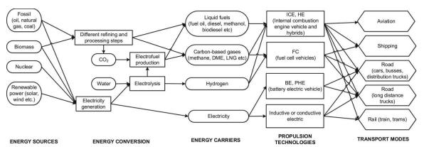
Figure 2. Potential pathways implying PtX processes (source (Brynolf et al., 2018)\*)
