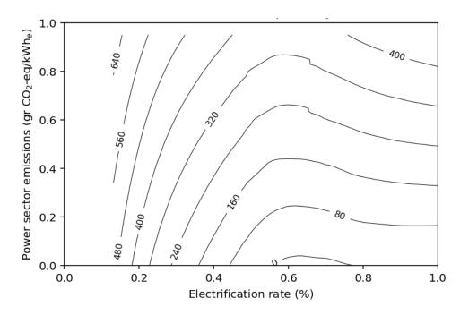
**Figure 30.** Contour plots of total emissions of the primary energy (Mt CO<sub>2</sub>) needed to satisfy the heating demand for different degrees of electrification and power sector decarbonisation
