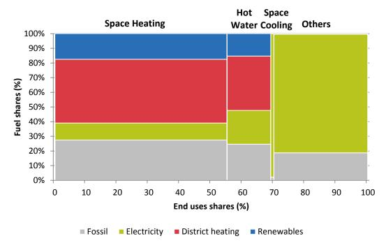
**Figure 45.** A comprehensive view of useful composition of the built environment for different uses and fuels in the EU. based on the current CHP full potential scenario
