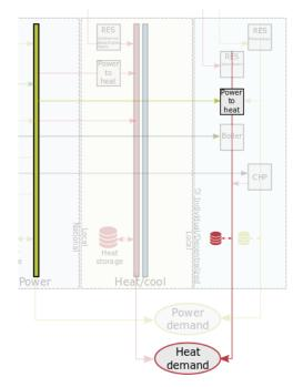
Figure 26. Focus on "electrification of heating" decarbonisation pathway. See Figure 21 for the whole picture
