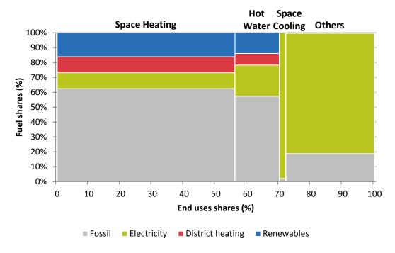
Figure 3. A comprehensive view of useful energy composition of the built environment for different end uses and fuels in the EU
