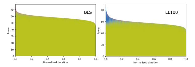
**Figure 59.** Aggregated flexibility needs (GW) in the form of a load duration curve for (left) BLS (right) E100. Colour coding: Green (outflows) blue (storage), red (curtailment)
