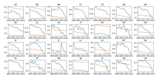
**Figure 29.** Tons of CO<sub>2</sub>-emissions per MWh of useful heat provided by heat pumps (blue) in comparison to conventional gas boilers (orange).
