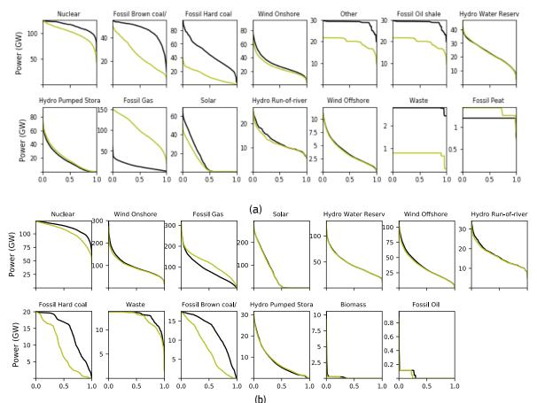
(b) **Figure 75.** Power plant generation per technology for the base case scenario (black) and the full potential CHP and thermal storage (green) in the form of Load duration curves for (a) 2016 and (b) 2050
