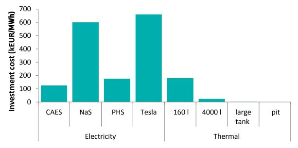
**Figure 35.** Investment cost per unit of stored capacity of electric and thermal storage options (Østergaard et al. 2016)
