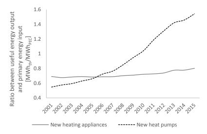
Figure 31. Performance with regard to primary energy consumption of heat pumps in comparison to the average new heating appliance in the EU28's residential sector
