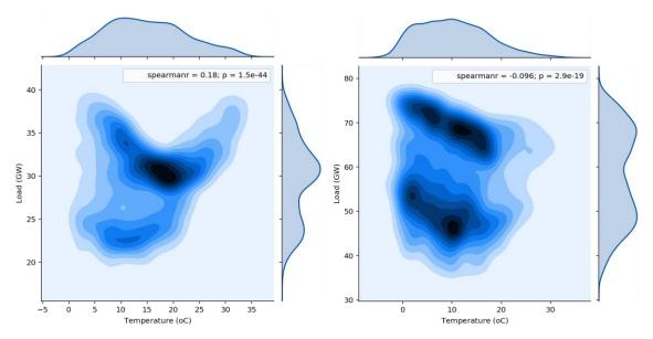
**Figure 17**. Density scatterplots illustrating the relationship between load and temperature for Spain (left) and Germany (right). The marginal distributions of the two variables are also shown to indicate the bimodal nature of the load (daynight, weekend-weekday).
