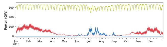
Figure 18. Aggregate electricity demand for heating (red) cooling (blue) and other purposes (green) in 2016. NB: Lines are not plotted cumulatively
