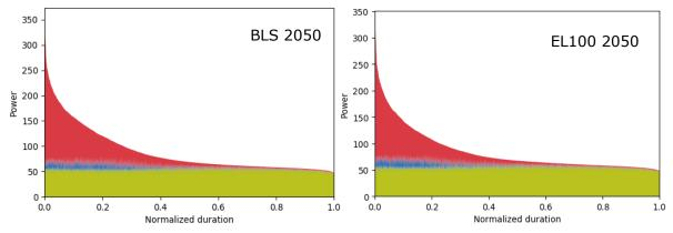
**Figure 66.** Aggregated flexibility needs in the form of a load duration curve for (left) BLS 2050 (right) EL100 2050. Colour coding: Green (outflows) blue (storage), red (curtailment)
