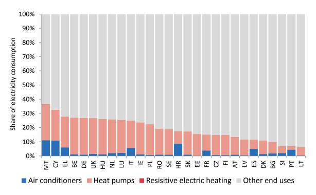
**Figure 38.** Heating and cooling share of electricity demand per Member State in a full heat electrification scenario EL100 (based on 2015 demand) (excluding process heat and cooling)
