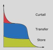
**Figure 50.** Conceptual merit order of flexibility represented as duration curve
