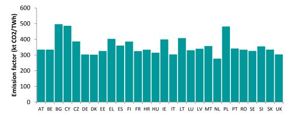
Figure 10. Emissions factors of the heating sector (space and hot water for residential and tertiary sector) in 2015 per unit of useful energy. Electricity and district heat are not accounted.
