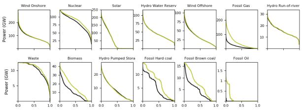
Figure 64. Power plant generation per technology for the base (BLS2050) and the full electrification case (FES2050)
