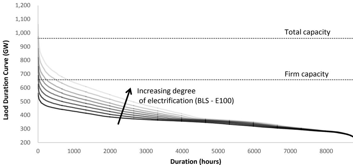
**Figure 39.** Load duration curve for different electrification scenarios. Today's firm and total power generation capacity is presented for reference.
