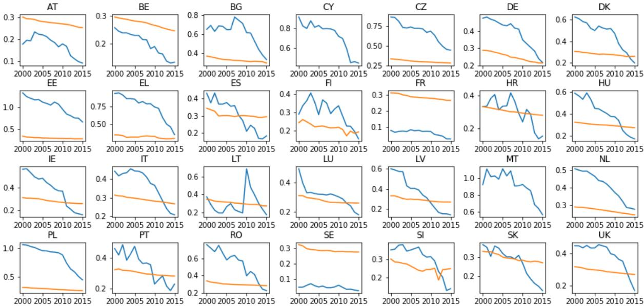
**Figure 29.** Tons of CO<sub>2</sub>-emissions per MWh of useful heat provided by heat pumps (blue) in comparison to conventional gas boilers (orange).
