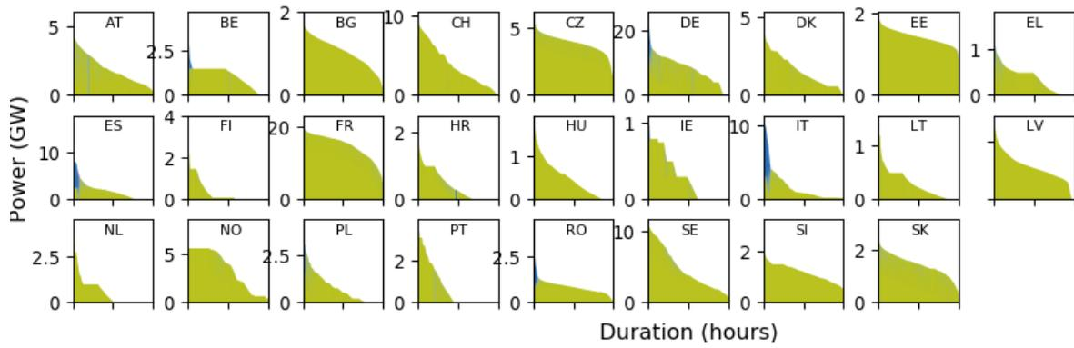
**Figure 58.** Flexibility needs in the form of a load duration curve for E100. Colour coding: Green (outflows) blue (storage), red (curtailment)
