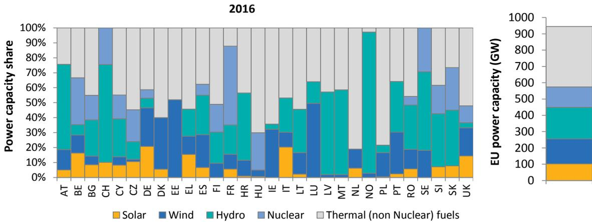
**Figure 22.** Power generation capacity and technology shares for today's EU (plus NO and CH) power system
