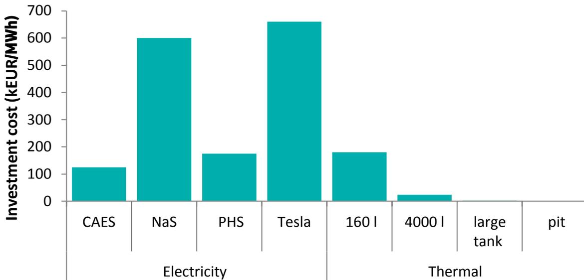
**Figure 35.** Investment cost per unit of stored capacity of electric and thermal storage options (Østergaard et al. 2016)
