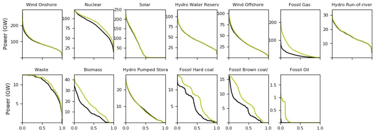
**Figure 64.** Power plant generation per technology for the base (BLS2050) and the full electrification case (FES2050)
