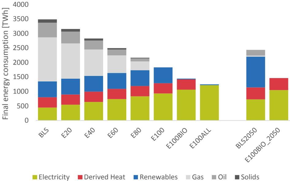
**Figure 36.** Final energy consumption for space heating in EU for different electrification scenarios
