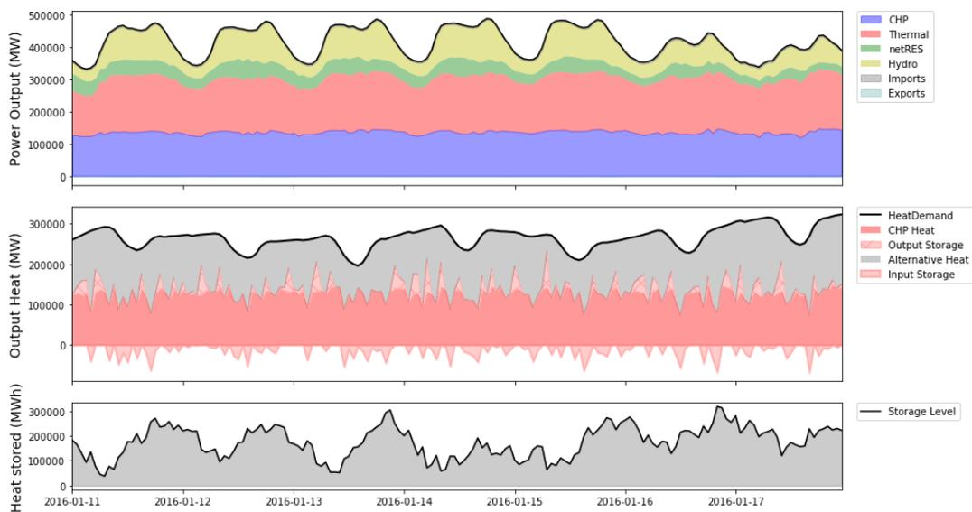
**Figure 92.** Heat and power. Full potential CHP and thermal storage scenario
