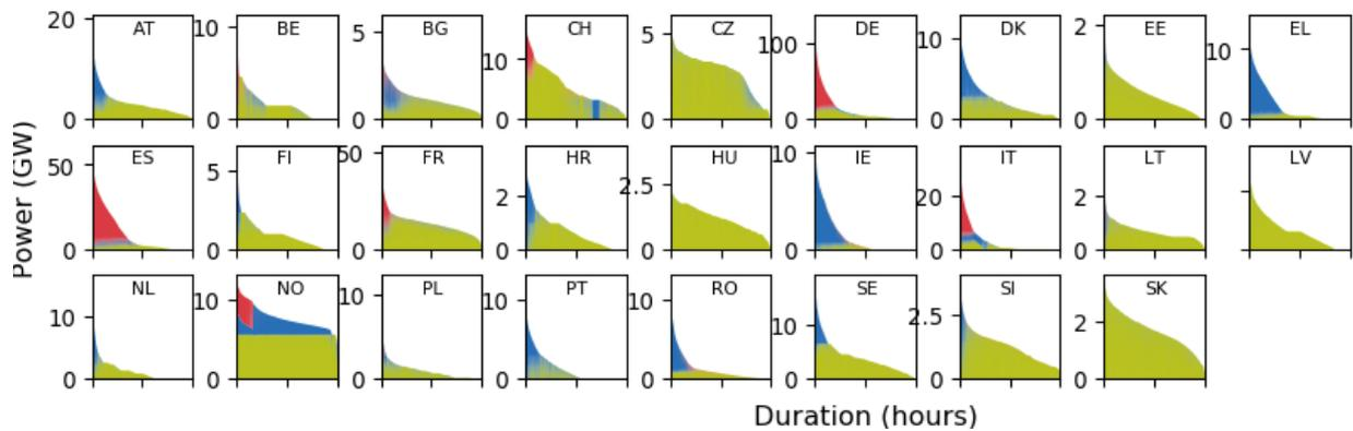
**Figure 65.** Flexibility needs in the form of a load duration curve for E100 2050 scenario. Colour coding: Green (outflows) blue (storage), red (curtailment)
