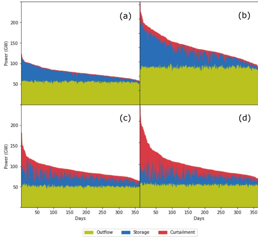
**Figure 78.** Flexibility options for different scenarios: (a) Base case 2016, (b) full CHP potential + thermal storage for 2016, (c) Base case 2050 and (d) full CHP potential + thermal storage for 2050.
