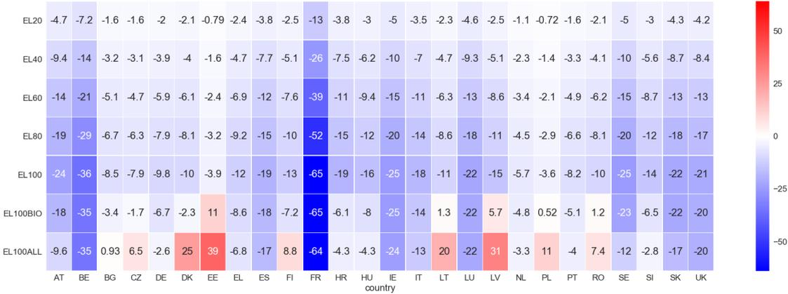
**Figure 56.** Change in CO<sub>2</sub>-emissions (%) in the power and the heat sector combined in the different electrification scenarios compared to BLS
