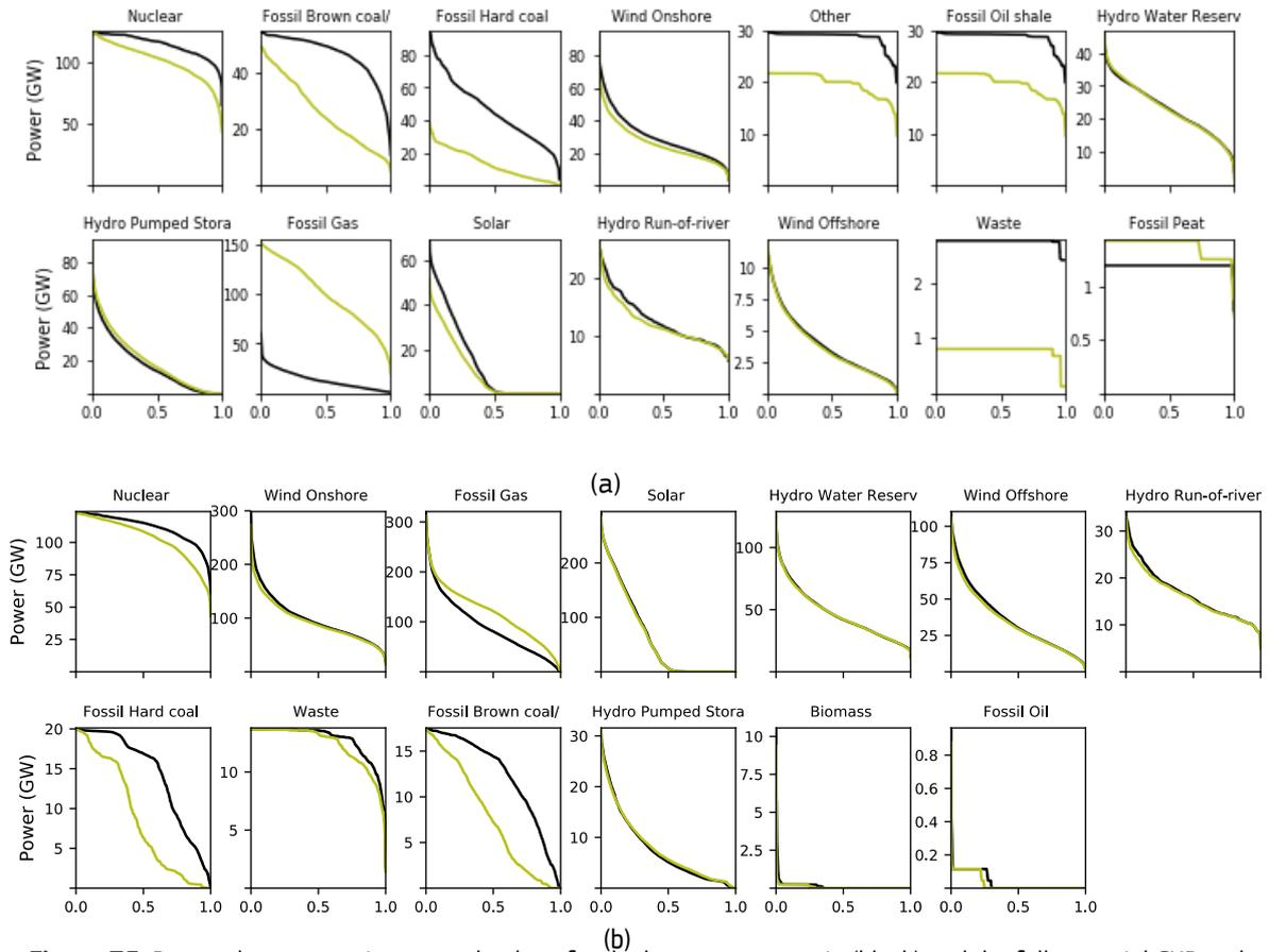
**Figure 75.** Power plant generation per technology for the base case scenario (black) and the full potential CHP and thermal storage (green) in the form of Load duration curves for (a) 2016 and (b) 2050
