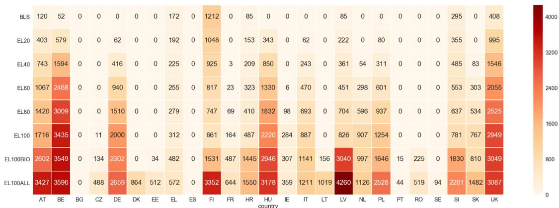
Figure 52. Number of hours during which the demand for electricity exceeds the firm capacity level, per Member State and scenario. Luxembourg excluded due to its strong import dependency, which results in load always exceeding the firm capacities.
