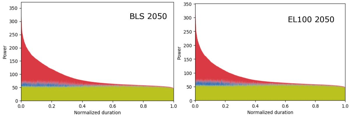
**Figure 66.** Aggregated flexibility needs in the form of a load duration curve for (left) BLS 2050 (right) EL100 2050. Colour coding: Green (outflows) blue (storage), red (curtailment)
