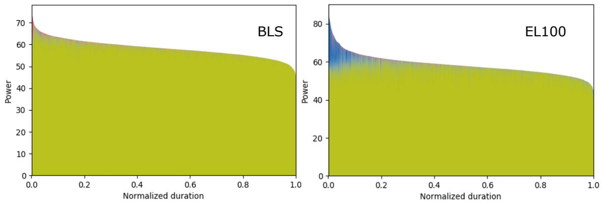
**Figure 59.** Aggregated flexibility needs (GW) in the form of a load duration curve for (left) BLS (right) E100. Colour coding: Green (outflows) blue (storage), red (curtailment)
