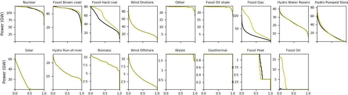
**Figure 57.** Power plant generation per technology for the base (BLS2015) in black and the full electrification scenario (E100) in green
