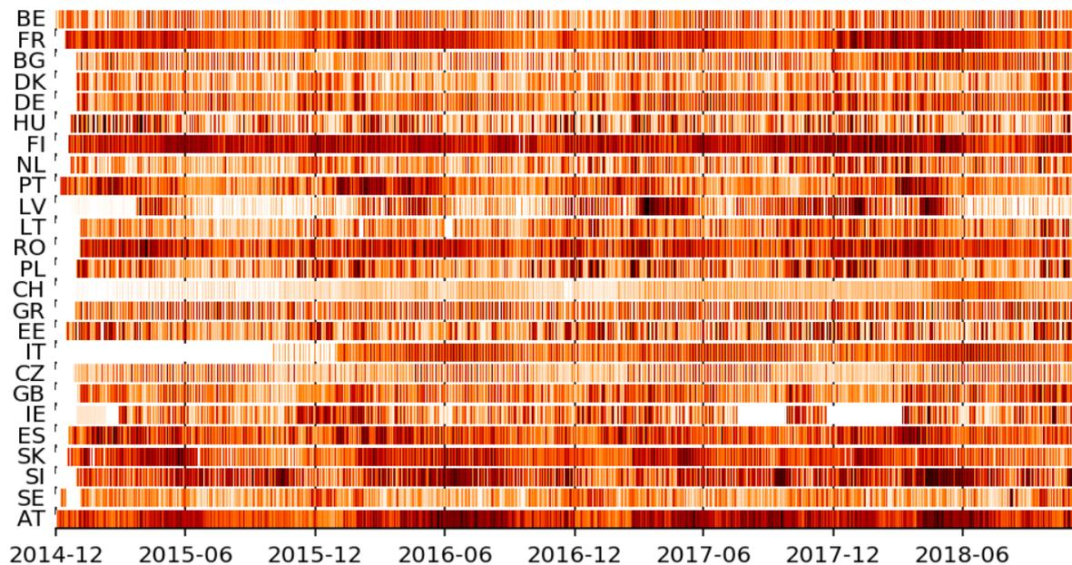
**Figure 84.** Variable renewable generation across EU. Data source: (ENTSOE 2018). The intensity of the colour corresponds to power generation from variable energy sources (the darker the colour the more energy is generated)
