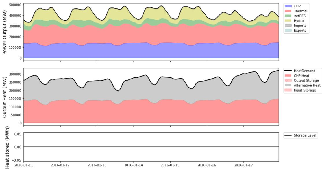
**Figure 91.** Heat and power dispatch. Full potential scenario with no thermal storage
