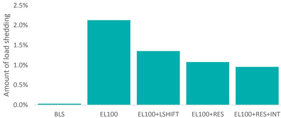
**Figure 67.** Load shedding sensitivity to additional renewable generation, interconnections and load shifting in the EL100 scenario
