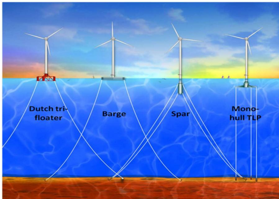
Figure 6 Most common offshore floaters.
