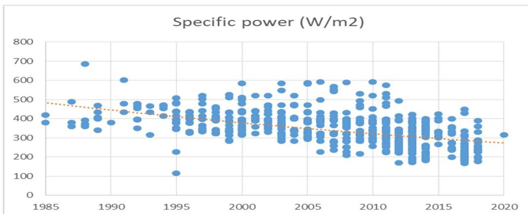
Figure 2 Trend to lower specific power in turbine prototypes. Turbines with lower specific power sweep larger areas for the same electric rating. Source: JRC database.
