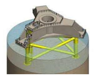
Figure 8 Three-legged jacket foundation with concrete transition piece. Courtesy Siemens
