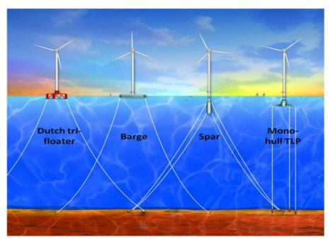
Figure 6 Most common offshore floaters. Drawing courtesy Floating Wind Turbines [91]
