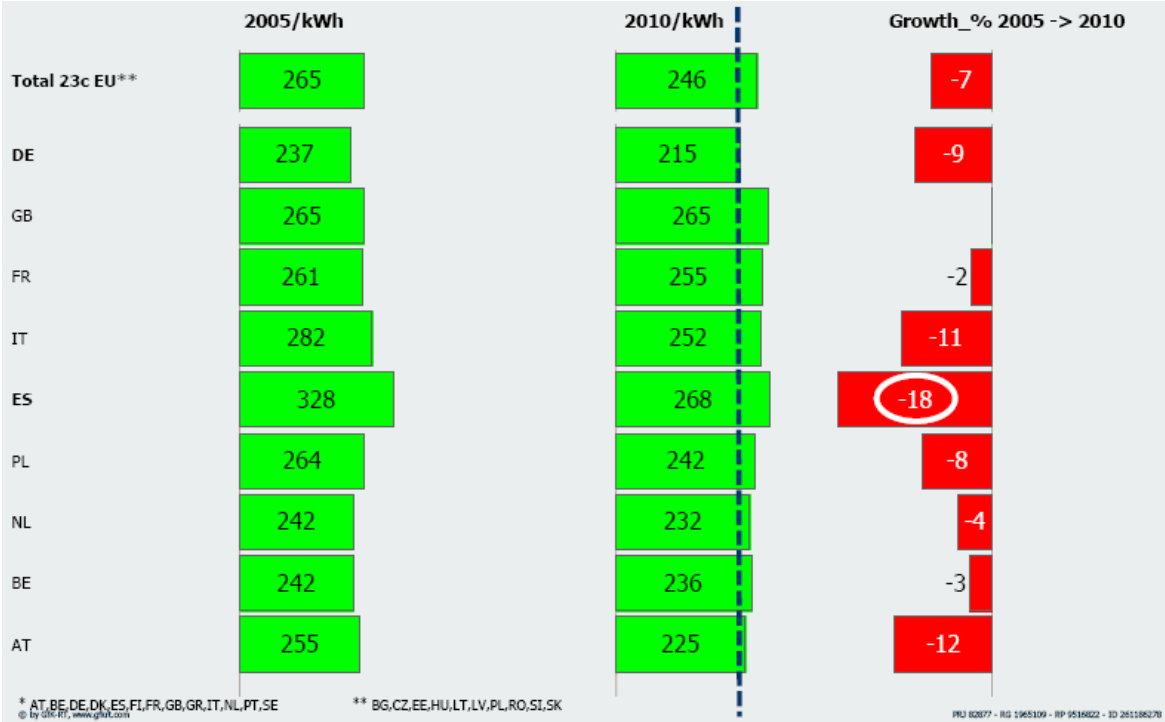
Fig. 33: Sales-weighted average annual energy consumption of MDA 4 7 in major EU markets (source GfK)
