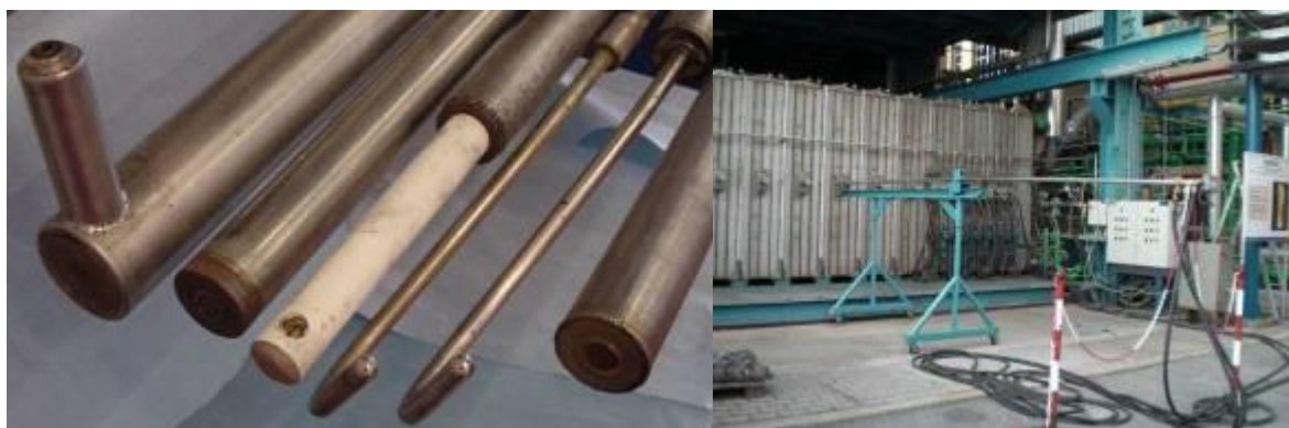
IFRF probes for in-flame measurements in FO.SPER
