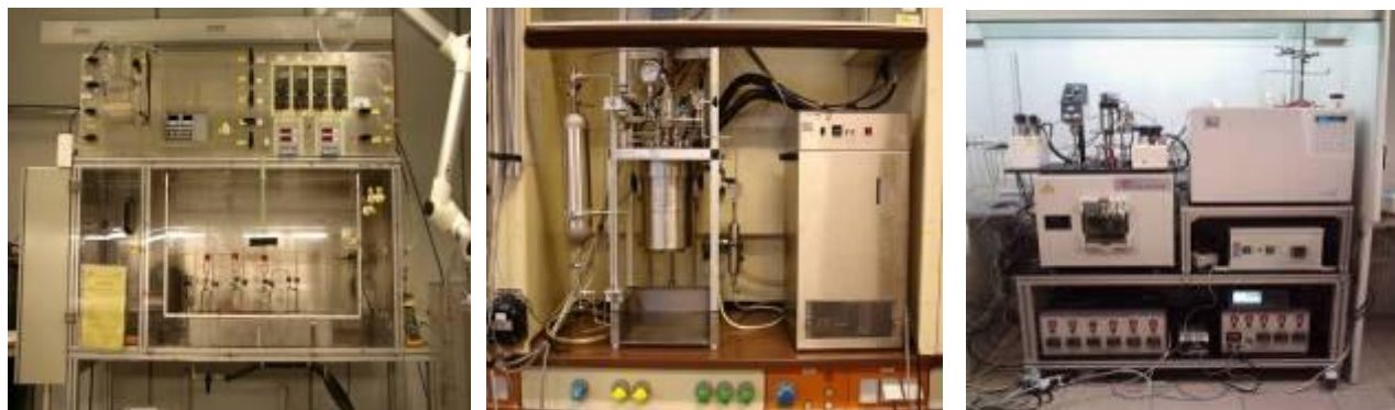
Figure 1. Pictures of low pressure VLE apparatus (left), reactor calorimeter (middle) and high pressure VLE apparatus (right).
