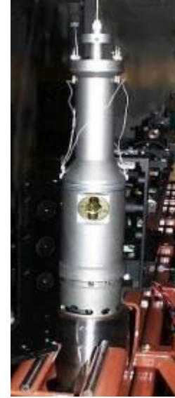
Fig. 4: Fluid cell for IFT-measurements (working conditions: 700 bars and 180 °C)
