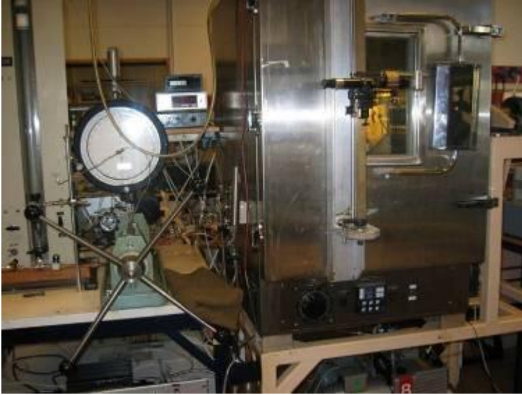
Fig. 3: Fluid pVT equipment (working conditions: 700 bar and 150 °C)
